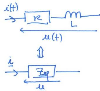
$$\text{Ainsi } \underline{u} = \underline{Z}_{ep} \underline{i} \Rightarrow \underline{U} = (R + jL\omega) \underline{I}$$
