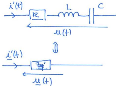
$$\begin{aligned} \underline{Z}'_{ep} &= R + jL\omega + \frac{1}{jC\omega} \\ &= R + j\left(L\omega - \frac{1}{C\omega}\right) \end{aligned}$$
