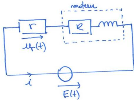
$$\text{Ainsi } U = |U e^{j\varphi}| = \left| \frac{rE}{r + R + jL\omega} \right| = \frac{rE}{\sqrt{(r+R)^2 + (L\omega)^2}}$$
