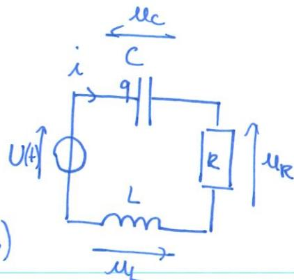
Or  $u_C = \frac{q}{C}$ ,  $u_R = R.i = R \cdot \frac{dq}{dt}$  et  $u_L = L \frac{di}{dt} = L \frac{d}{dt} \cdot \frac{dq}{dt}$
