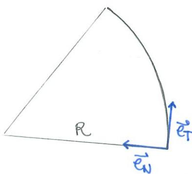
$$\text{Donc : } \vec{a} = \frac{v^2}{R} \vec{e}_N \quad \text{et} \quad \|\vec{a}\| = \frac{v^2}{R} = \frac{V_0^2}{R}$$
