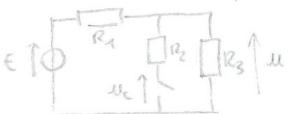
$i_2 = i_3 = \frac{E}{R_1 + R_3}$  et  $u = u_c$
